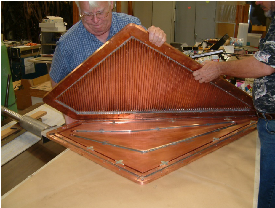
Fig. 1. The K150 cyropanel during its construction.
